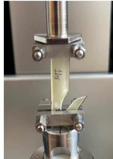
Figure 5 UVO exposed then shape recovered sample broken after loading in DMA.
