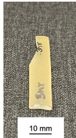
Figure 2 UVO treated sample after shape recovery develops curvature on the end.
